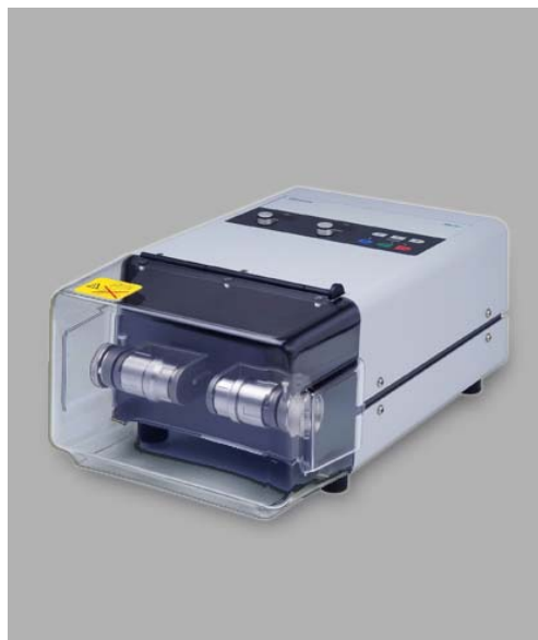
Figure 9: Mill with a ZrO_2 grinding vessel for grinding of up to 10 g.
