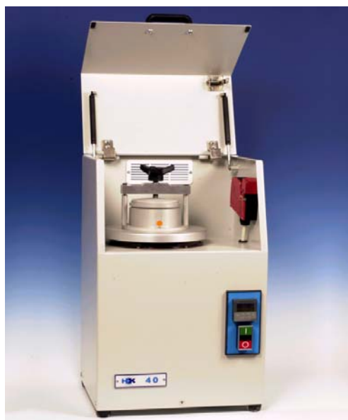
Figure 10: Mill with an Al_2O_3 grinding vessel for grinding of up to 60 g.
